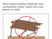
Avoid accidents by following these important guidelines 1. Brace and nail each I-joist as it is installed, using hangers, blocking panels, rim board, and/or cross-bridging at joist ends. When I-joists are applied continuous over interior supports and a load-bearing wall is planned at that location, blocking will be required at the interior support. See APA Builder Tips: Blocking for I-Joist Systems, Form
