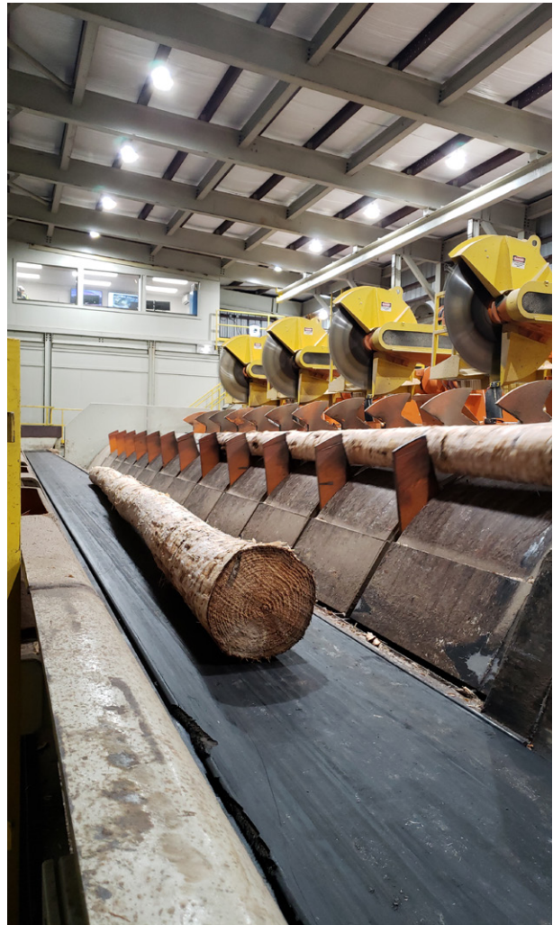
This new log merchandiser, installed at Monticello in 2019, determines the optimum length to buck each log to maximize value.
