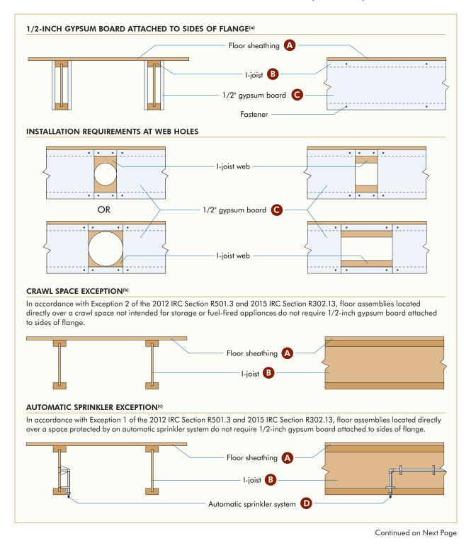
A Floor sheathing: Materials and installation in accordance with the 2012 and 2015 IRC Section R503.
