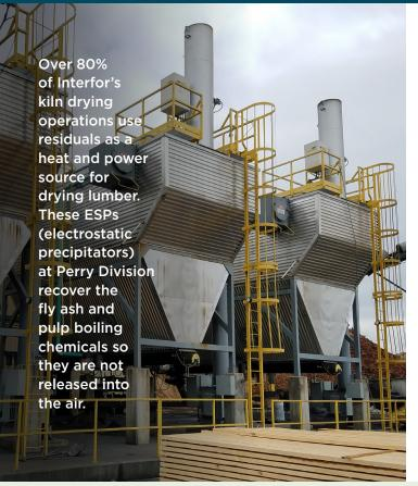
Over the years Interfor has made significant investments in its manufacturing facilities that improve sawmilling efficiency, reduce energy consumption, and reduce GHG for processing, drying and transporting lumber.
