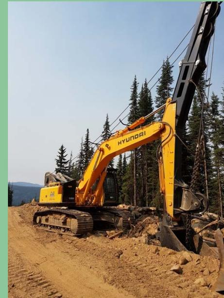
The Adams Lake operation has implemented innovative harvesting systems—traction line and tether systems—on steep slopes to increase operator safety and allow the retention of trees rather than a full clearcut.
